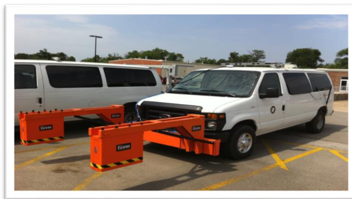
Figure 1. AHTD Air-Coupled GPR Unit
